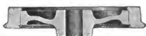
Figs. 4555-4556. No. 14 Krupp Wheel. Patent Wrought Iron Disc Center. Steel Tire Secured with Bute Fastening.
